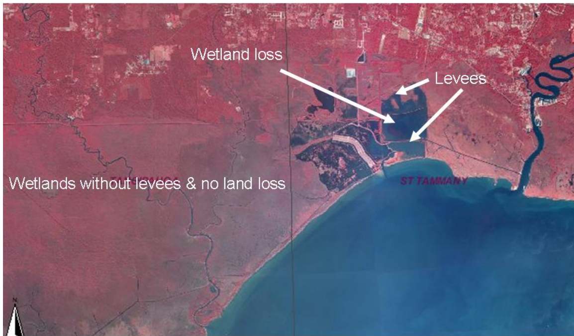
Figure 4: Example of wetland loss due to levee construction around wetlands. Land has subsided due to lack of plant growth creating unnatural “square lakes” along old levee alignments. Note adjacent areas (east and west) without levees are solid wetlands.
